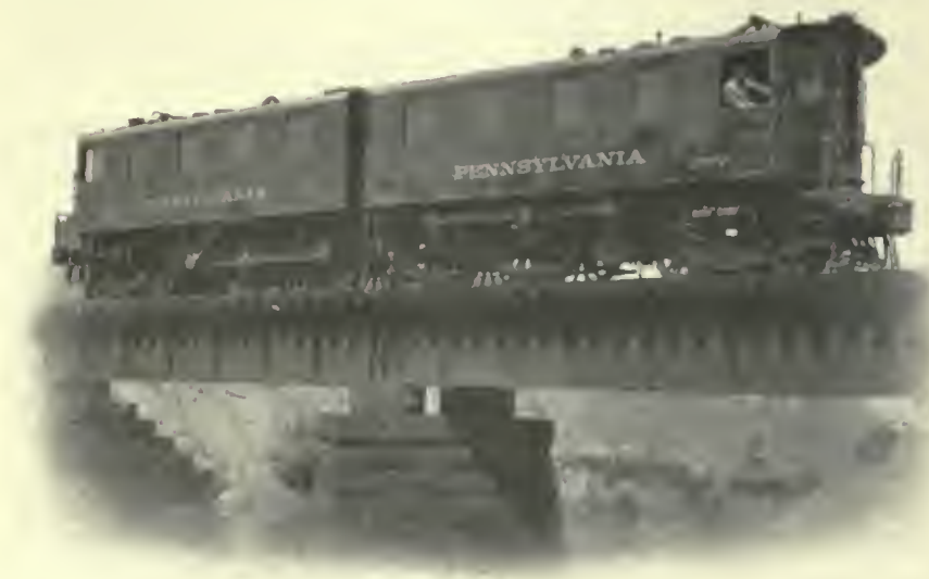
FIG. 533. ELECTRIC LOCOMOTIVES. Electric Locomotive for 600-Volt Direct Current Third Rail Operation, Pennsylvania Railroad.
